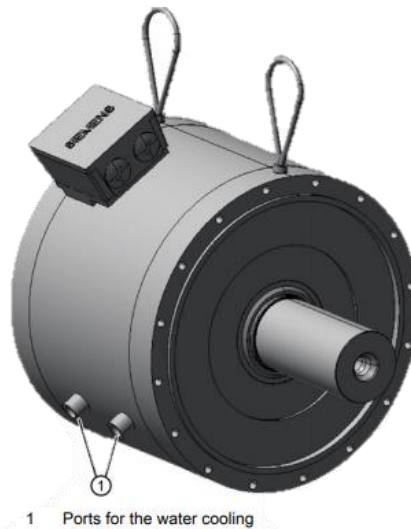
Figure 15. Generator cooling ports [3]
